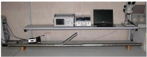
Designed to determine the bulk density of rocks in open-hole or cased with a plastic pipe wells of small
