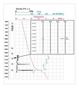
\$\triangleq \text{ Accordind to EMDS-S data interpretation more than 20 local defects- corrosion pits 0.9-13 cm3 in volume are revealed in injection point № 529 with the interval of 1060-1350 m
