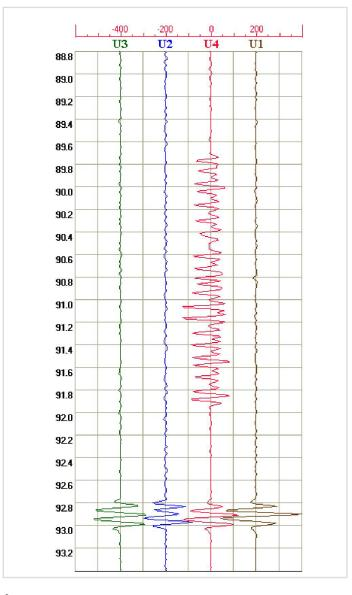
♦ Monitor well NPF «Geophizika». EMDS-S defectoscope clear fixates all 21 holes, which were drilled by PS-112 perforator. All the holes are drilled on the one side of the column, that's why it is fixated only by one sonde of small defects
