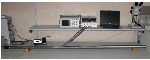
Designed to measure the effective atomic number Z of rocks in open hole well, to identify ore intervals with anomalous Z, and to determine the ash content of coal seams.
