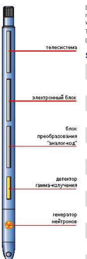
Designed to determine the elemental composition of rocks in ore wells by measuring the full gamma radiation spectra of radiation capture of elements, which are part of rocks and ores, when they are irradiated with fast neutrons using a pulsed neutron generator.
