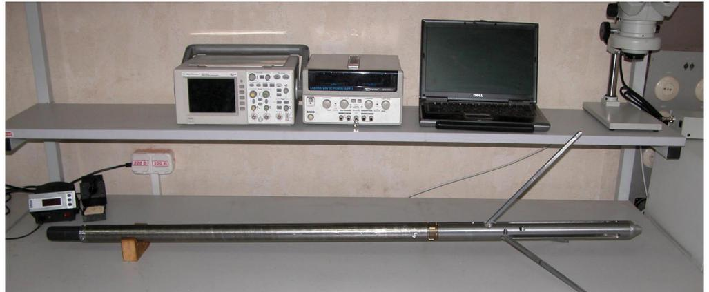
Designed to measure the diameter of ore, coal and hydrogeological wells.
