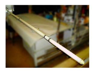
Designed for simultaneous measurement of apparent electrical resistance (a), spontaneous polarization potential (SP), exposure dose rate (EDR) of gamma radiation with a quantum energy of 0.03-3 MeV (GR).
