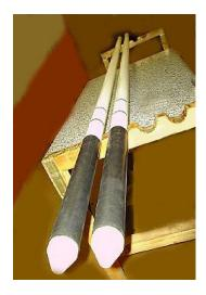
Designed for simultaneous measurement of apparent electrical resistance (a) with switching the configuration of the sondes (lateral sonde-normal sonde) with simultaneous and forced switching of the sondes configuration, as well as spontaneous potential (SP) and exposure dose rate (EDR) of gamma radiation in uranium deposits wells. At the request of the customer, it can be equipped with a magnetometric inclinometer module (modification KSP-GK-43I).
