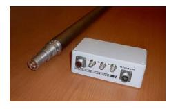
The LOM-2 processor Overhauser magnetometer is a precision measuring tool based on the principle of dynamic polarization of nuclei (Overhauser effect), intended for measuring the module of the Earth's magnetic field induction. The magnetometer is based on an Overhauser nuclear precession converter with a stable working substance (lifetime is about 3-5 years). By compared to proton converters, this type of converter has lower power consumption, greater sensitivity and gradient stability.
