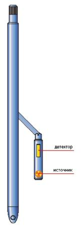
Designed to measure full spectra of characteristic X-ray radiation of atoms of elements that make up the rocks and ores during the logging of ore, coal, hydrogeological and special wells. The tool provides quantitative determination of chemical element contents in formations intersected by wells.
