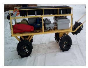
SPO-P-500Sh round-trip equipment is designed for round-trip operation during geophysical surveys of wells drilled in mine workings hazardous for gas and oil for exploration of solid mineral deposits.
