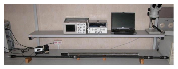
Designed to measure the effect of induced polarization (IP), apparent resistivity (AR), spontaneous polarization potential (SP) and exposure dose rate (EDR) of gamma radiation of rocks during the study of geological exploration wells.
